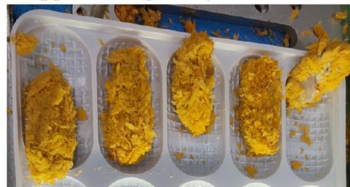
Gripper 2, 16 g, 90 oysters/min, 45°
