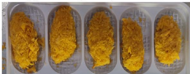
Gripper 2, 16 g, 90 oysters/min, 0°
