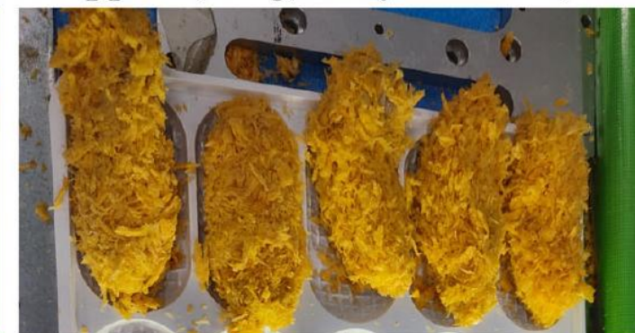
Gripper 2, 40 g, 90 oysters/min, 0°
