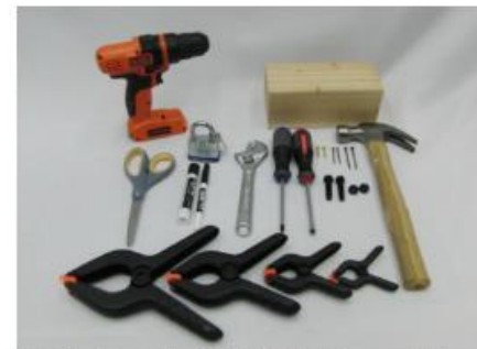
Fig. 3: Tool items in the YCB Object Set: back: power drill, wood block; middle row: scissors, padlock and keys, markers (two sizes), adjustable wrench, pliers and flat screwdrivers, wood screws, nails (two sizes), plastic bolt and nut, hammer; front: spring clamps (four sizes)
